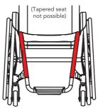
(The tilt adjustable footplate only is suitable with the V shaped front frame)
